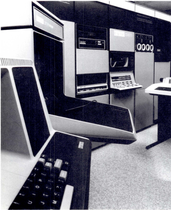
Above: The new XVM versions of Digital's 18-bit PDP-15 are used extensively in computer-aided design applications; graphics features add to its interactive design capabilities.
